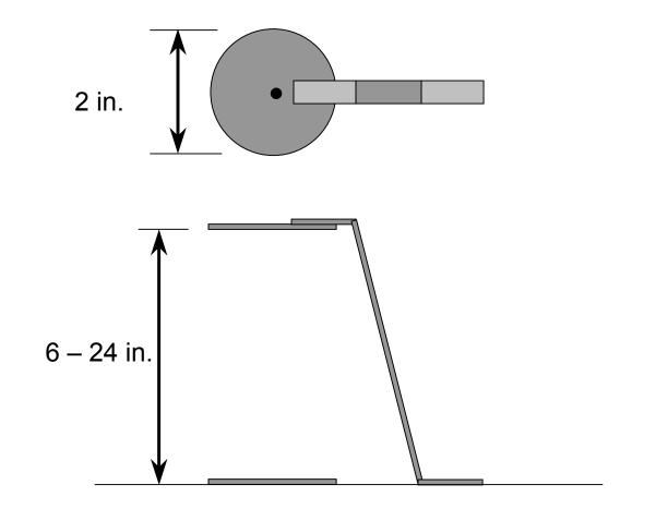
The mirror must be attached to a surface guaranteed parallel to the Elevation or Roll axis while perpendicular to the Azimuth or Tilt axis.
